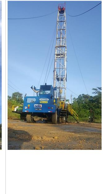
**RIG #3** Description: Pole Rig Woodfield- Double Pole 55 ft. Mast Hook Load 60,000 lbs.
